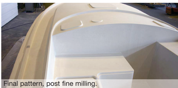
Final pattern, post fine milling.
