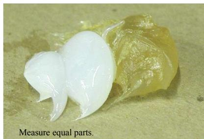
**Mixing:** Mix 1 part resin to 1 hardener by volume. Mix with a palate knife or spatula until uniform in color. Magic-Smooth is tolerant of slight variations. You can mix as little or as much as possible but be careful not to mix more than you can use within the working time or you will end up with wasted material once it starts to cure and becomes unusable.
